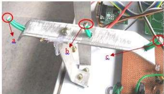
Fig. 3. Light Sensors. (a), (b) Side light sensors, (c) Middle Light Sensor
